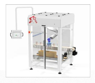
Our new design using machine vision to guide robots. Each robot equipped with automatic tool changer, that allow job change in less than 1 minute.
