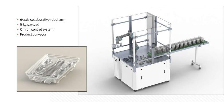
The system is designed to pack formed wire into pre-formed plastic packaging. This design allows autonomous production for up to four hours.
